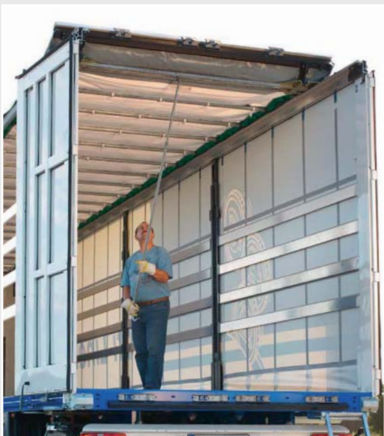
Tarpaulin bows for fixed and sliding rooftops of lorrys (Pictures: Krone).
