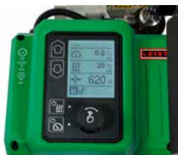
Digital display of welding pressure and voltage
